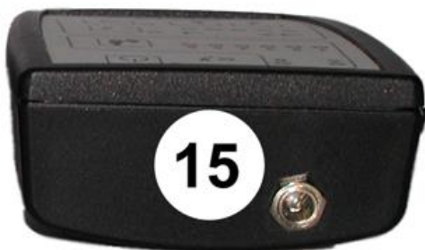
Figure 3.5: Charging connector on Misty Instructor Unit
